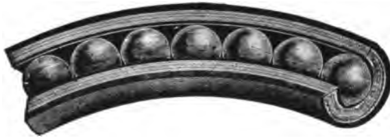
FIG. 106.—The Ball Tire. In this tire the ill effects of puncture are prevented by the solid rubber balls inserted in the tube, which transform the tire into a cushion, positively proof against flattening.
